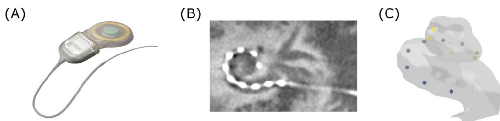
Figure: (A) Cochlear Implant (MED-EL, Austria) (B) Postoperative CT slice of the cochlear basal turn with CI electrodes (C) 3D visualization of the cochlea and electrode positions.
